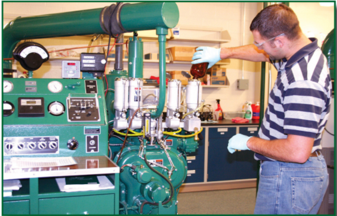
Lance Campbell pours fuel into a special four-horsepower engine that enables technicians to measure the octane level in the fuel.
