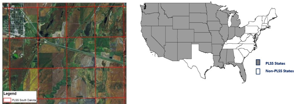
Figure 5: Grid concept close up of a specific area on the left. States covered under the PLSS layer on the right.
